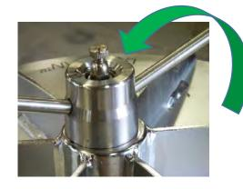
2. Open **VENT VALVE** (top of press)
