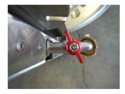
**5.** Begin to open inlet valve slightly to start the pressing.
