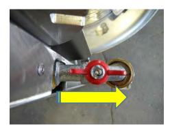
**3.** Open inlet valve all the way and the bladder will begin to fill.
