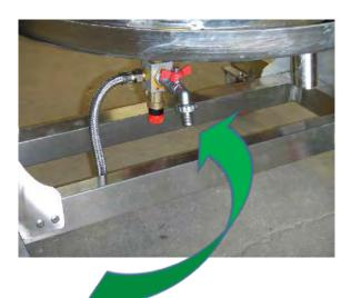
8. When the juice has completely finished flowing and the pressure gauge reaches 36-40 PSI, close the inlet valve and open the drain valve to empty the bladder. (on bottom of press).
